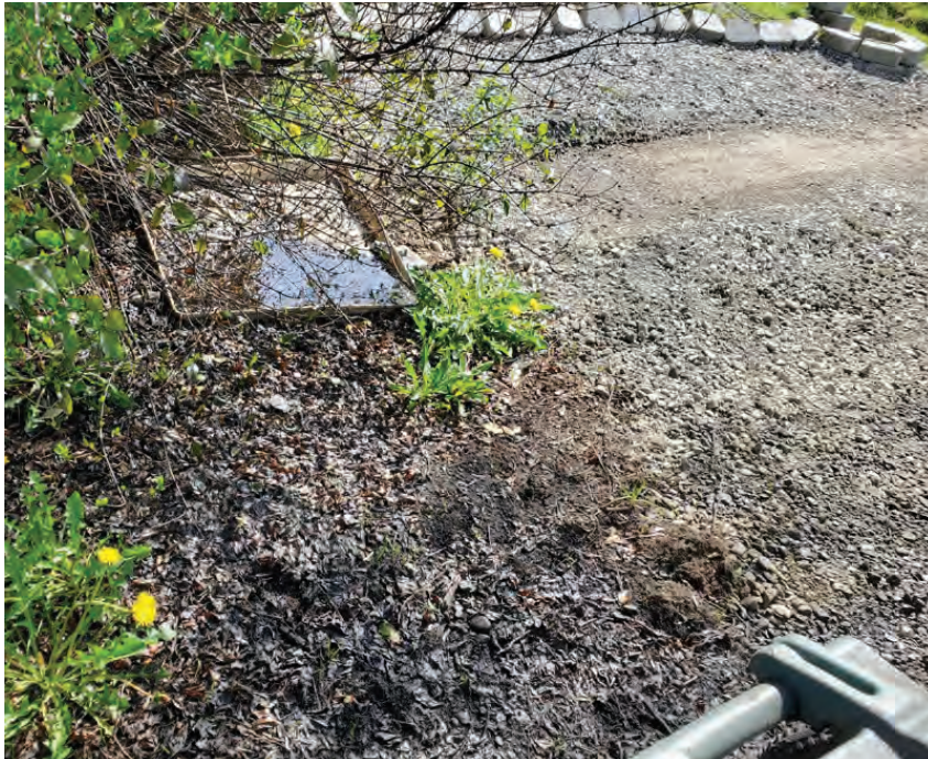
Figure 2 – Liquid oil in pan with no protection from the environment.
